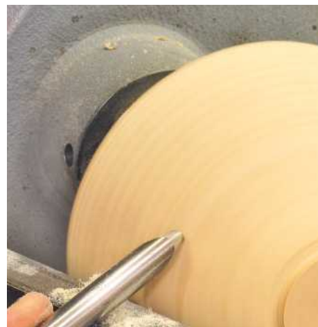
▲ Pic.6 Shear cutting with the gouge is a fairly modern technique. The handle is down and the lower cutting edge is presented with the flute almost closed off. The shaving should be really fine here
